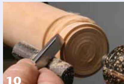
10 Use a skew chisel to clean up the endgrain.
