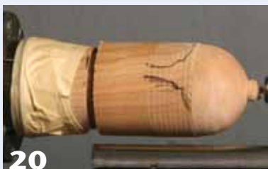
20 Using the tailstock for support, finish-turn the end of the lid.
