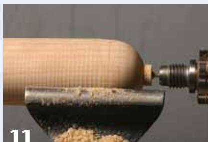
11 Fit the lid onto the cylinder, line up the grain, and bring up the tailstock.
