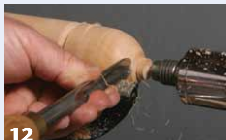
12 Shape the outside end of the first hemisphere aiming for a wall thickness of about 1/8" (3 mm).
