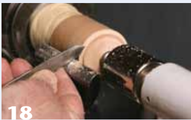
18 With the cylinder jam fitted onto the waste wood and the tailstock drawn up, turn a tenon on the end of the cylinder.
