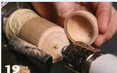
19 Fit the second hemisphere/lid onto the tenon.
