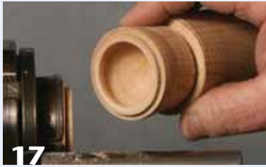
17 With a short waste-wood cylinder in the four-jaw chuck, turn a tenon to fit the inside of the hollow you created on the end of the second section.
