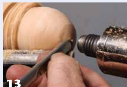
13 Slide the tailstock away and complete the hemisphere. Sand that end.
