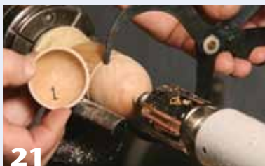
21 Use calipers to match the diameters of the two lids.
